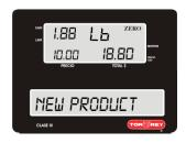
2.- Type in the Price of the new product and then place the product on the scale's plate, if you remove the weight off the scale the scale will go back to zero and the product's information would be gone.
