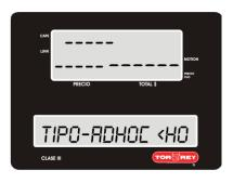
1.- Select the type of connection on the WLABEL scale. ADHOC<HOT SPOT> Following section **13.2.3**
