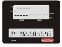
Select Network Info and look for the network's name and the ip address and sabe them to use them during the connection process. Your iOS device will use the scale's ip address as well as the nework's name to connect to it. On your iOS device select the network that your scale created.
