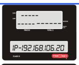
Shows the IP Address of the scale.
