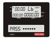
1.- Press the PROG button the word PASS will immediately appear in the advertising display: At this point, press the 123456 sequence and then press ENTER to enter the configuration menu.
