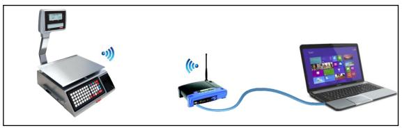
**The ETHERNET connection** is made with a network cable (RJ45) where you connect a modem, the scale and a computer
